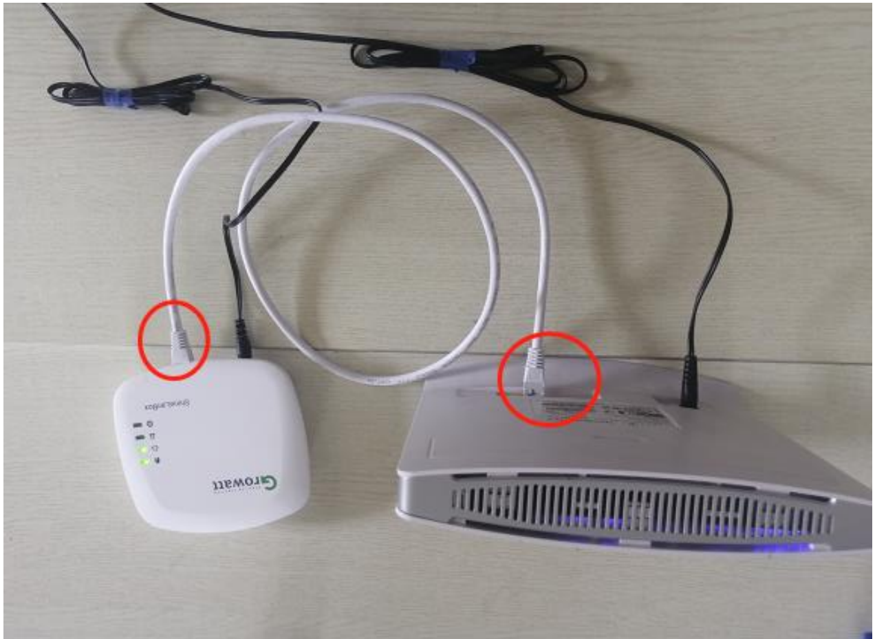
Figure3.communication line interface location
